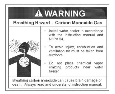
A gas water heater cannot operate properly without the correct amount of air for combustion, see Figure 9. Do not install in a confined area such as a closet, unless you provide air as shown in the *Locating The New Water Heater* section. Never obstruct the flow of ventilation air. If you have any doubts or questions at all, call your gas supplier. Failure to provide the proper amount of combustion air can result in a fire or explosion and cause death, serious bodily injury, or property damage.
